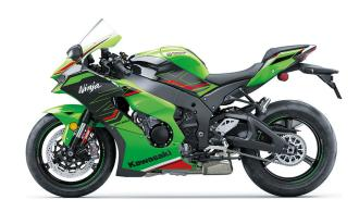
Brembo dual semi-floating 330mm discs with dual
